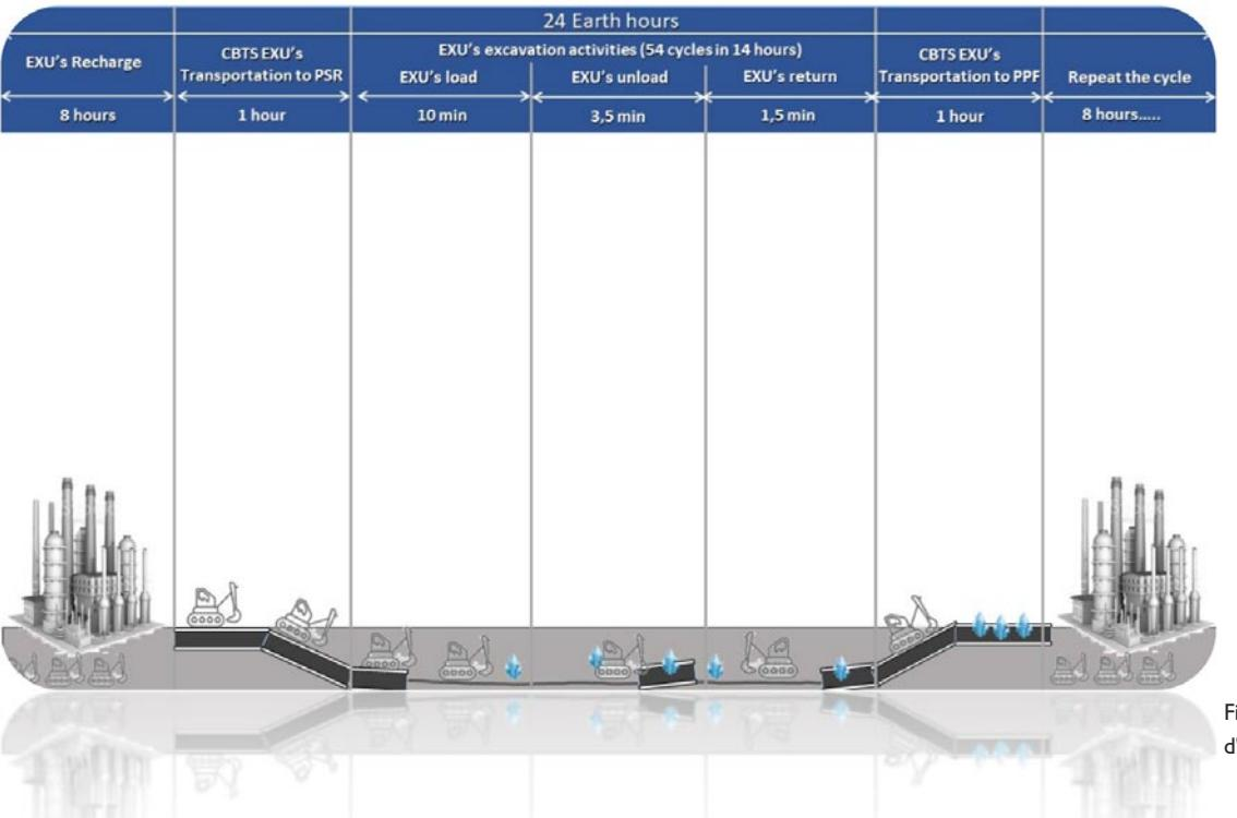
The resources extraction operations start with the swarm of EXU's located in the Propellant Production Facility, where the recharging operations are performed, which is close to the edge of the crater.
