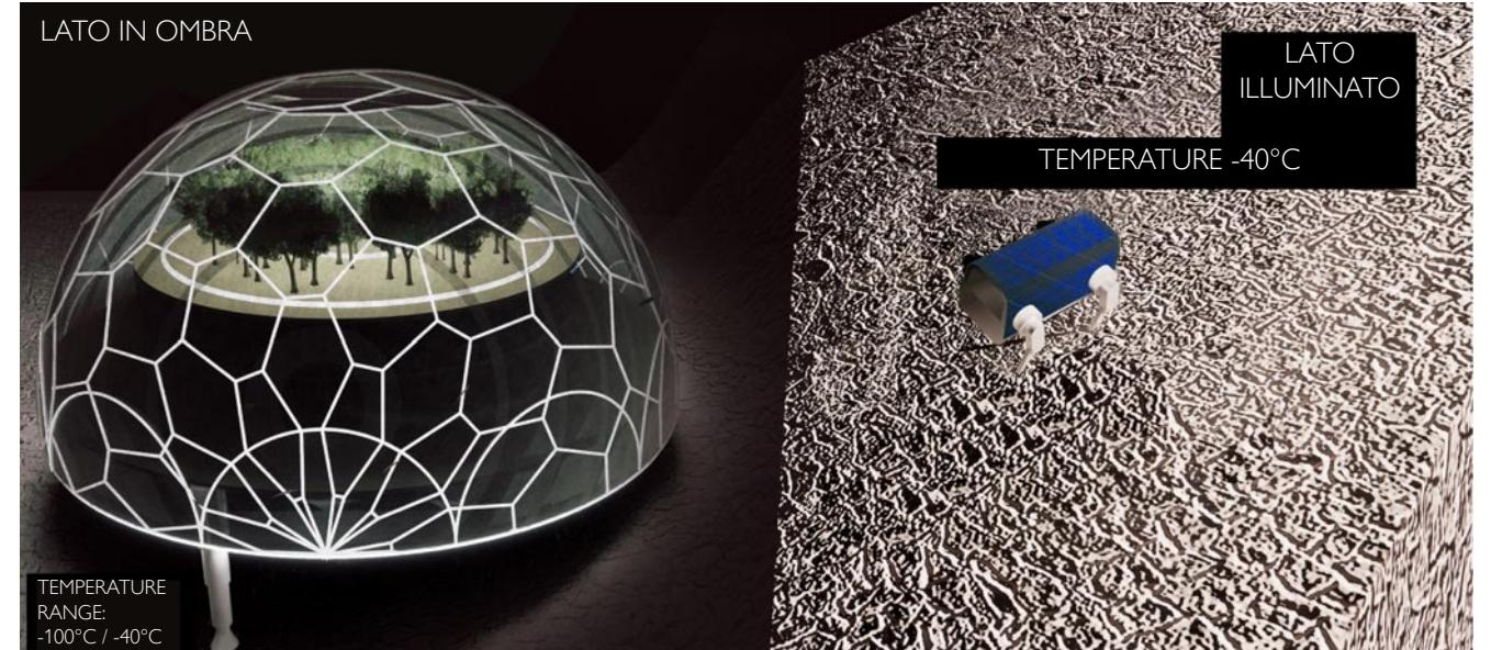
**The stable core** will grow over time without interfering with activities. Structurally, the hemisphere is based on a vertical connection (approx. 30 sqm) fixed to the ground and equipped for "lunothermics" and on 3 telescopic feet, capable of adapting to the complex elevation of the ground.
