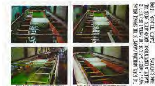
THE CONDUCTED HYDRODYNAMIC EXPERIMENTS DEMONSTRATED THAT 80% OF THE WAVE ENERGY WAS DISSIPATED WITHIN THE SPONGE BREAKWATER, 10% ONLY WAS REFLECTED BACK AND 10% WENT THROUGH. PERMEABLE SPONGE BREAKWATER - WAVE TRANSMISSION EXPERIMENTS.
